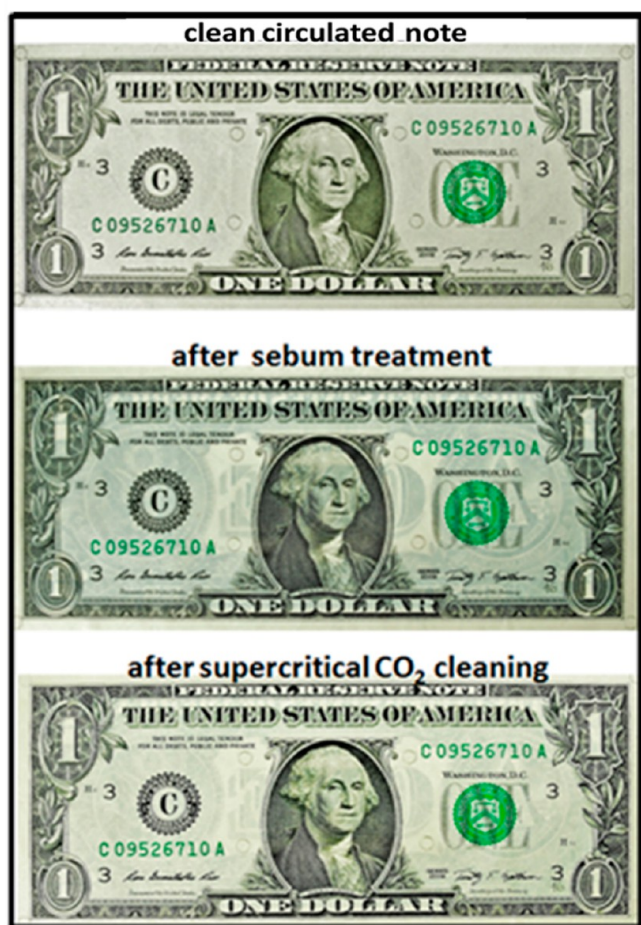
Figure 7. Banknotes before sebum treatment, after sebum treatment, and after cleaning with supercritical CO 2 at 60 °C with ultrasonic agitation.
