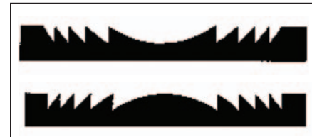
Two off-axis Fresnel lenses: negative focal length (top) and positive focal length (bottom)
