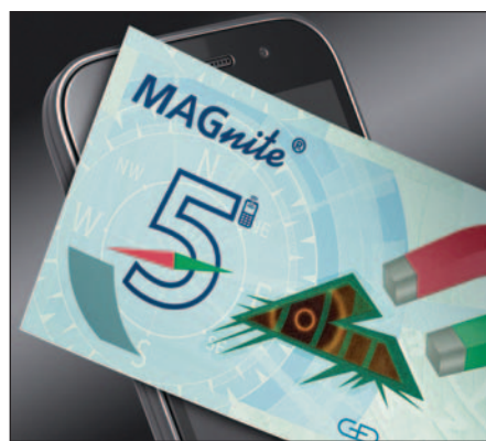
The magnetic field causes the pigments in MAGnite to become aligned and hence visible – as seen here by the shape of the speaker in the mobile phone behind the note, which appears in the printed MAGnite patch
